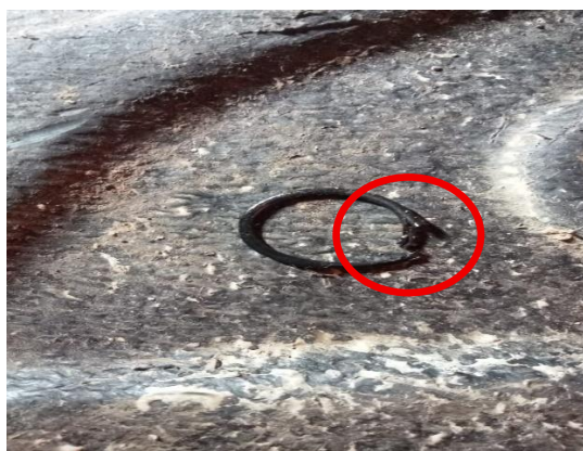
Gambar 4. O-Ring adapter hose oil cooler rusak
