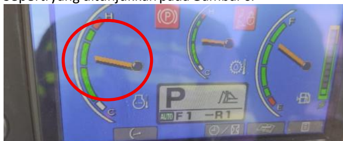
Gambar 5. temperature coolant mulai naik
