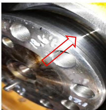
Gambar 3. Crankshaft contact with the seal
